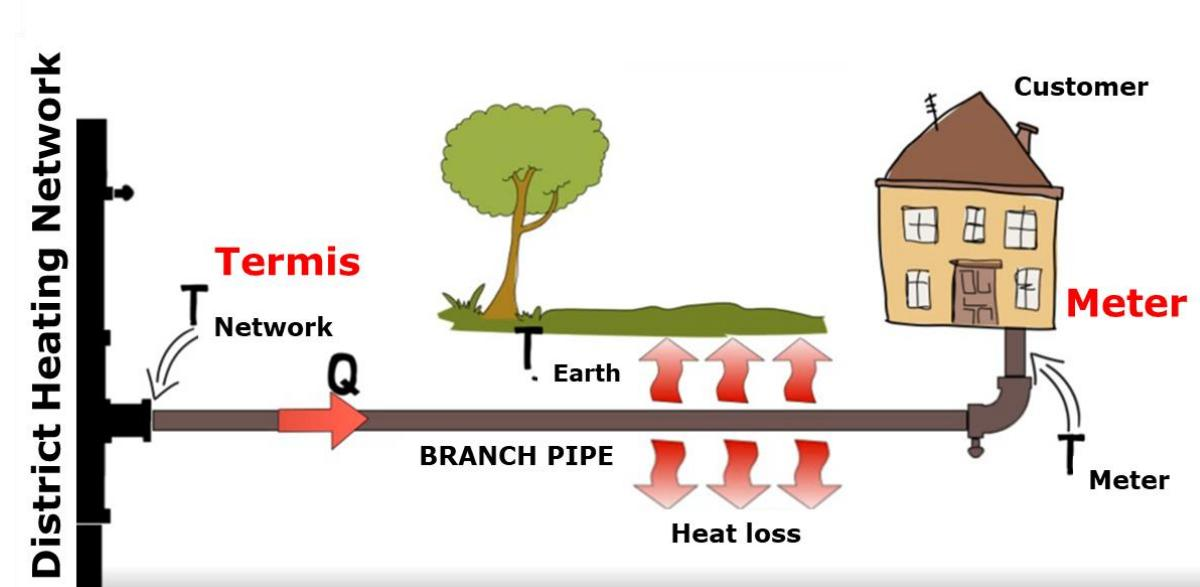
Figure 7. Principle diagram of the heat loss calculation tool
