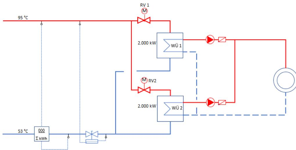
Figure 5: Exemplary substation for currently directly connected major customer
