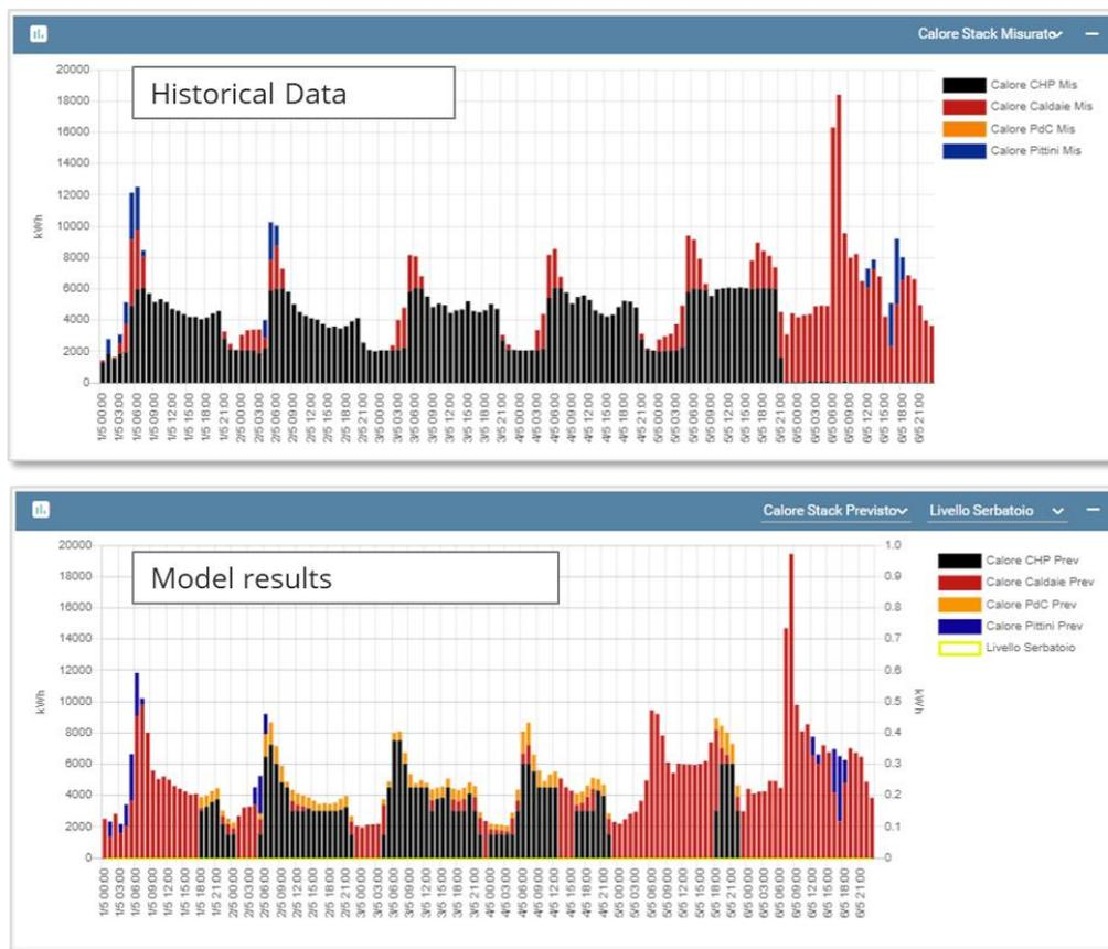
Figure 11: Comparison between historical data and model results showing the different use of CHPs
