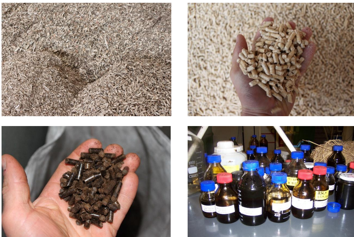
Figure 41: Typical biomass feedstock types for the use in DH: woodchips, pellets, torrefied pellets, pyrolysis oil (from top left to bottom right) (Sources: D. Rutz)
