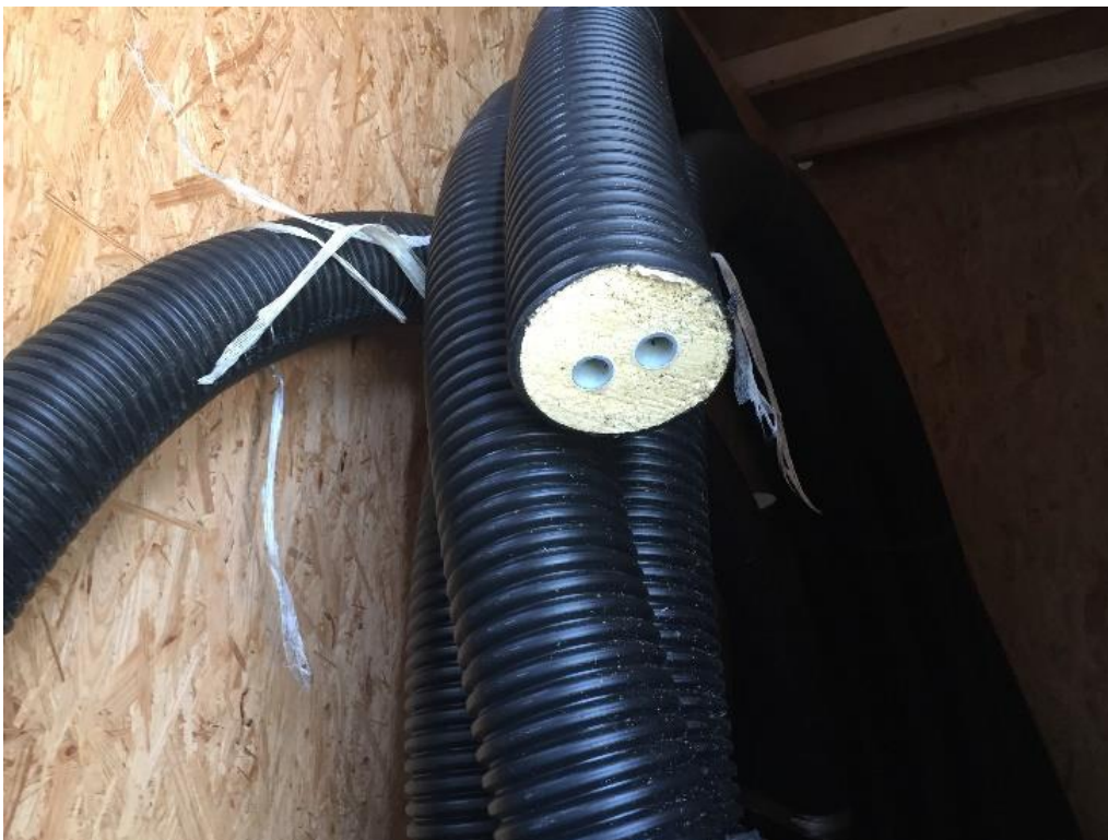
Figure 6: Low temperature DH enables the use of plastic piping (here a twin-pipe), which are less costly and due to its flexibility easier to mount (Source: B. Doračić)
