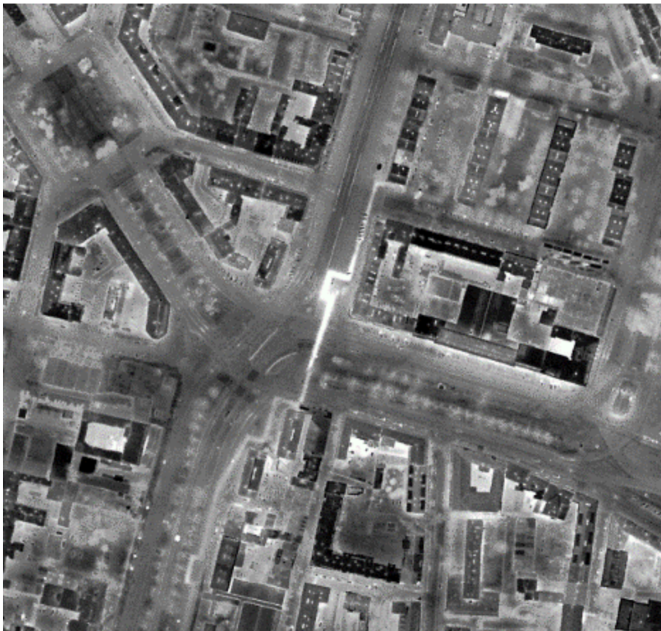
Figure 28: Thermal imaging via airplane (Source: SCANDAT GmbH)
