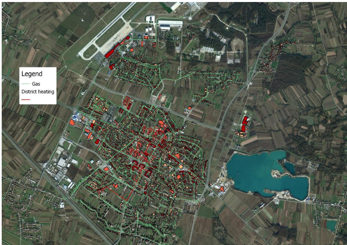
Figure 15. Natural gas and DH grid in the city of Velika Gorica in Croatia (Source: T. Novosel)
