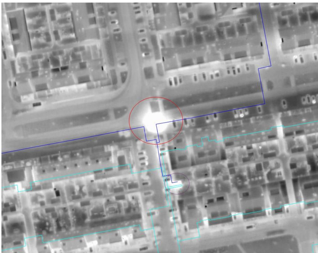
Figure 20: Thermal imaging of a DH network showing a major leak on a pipeline (Source: COWI)
